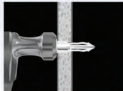
Insert anchor in hole and tap flush with wall.
